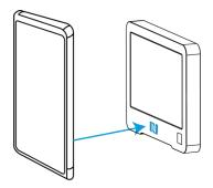
4. Basic information and settings of the device will be shown on ToolBox if it's recognized successfully. You can read and configure the device by tapping the Read/Write button on the App. In order to protect the security of devices, password validation is required when first configuration. The default password is **123456**.
