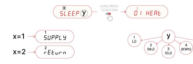
If a choice has not been made during the order, the meter must be configured. The configuration of the meter can be performed via buttons or via NFC through android app. If the activation takes place with buttons, the items in the menu will be two:
