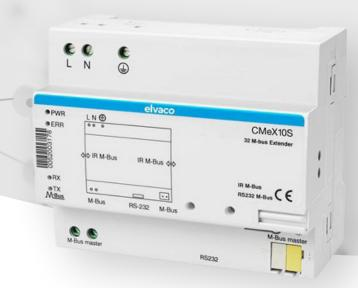
CMeX10S-13S is an M-Bus Master which, by providing additional drive strength, extends the number of meters an Elvaco CMe Series Gateway is able to use. The product is equipped with a unique IR Pass Through feature which enables up to four CMe/CMeX Series devices to communicate via IR, by stacking them side-by side. The product also supports integration with existing M-Bus systems through RS232.
