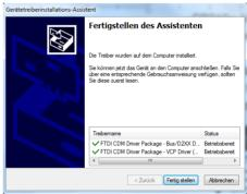
Now you can connect the PC. The USB driver for the PW100 is installed automatically and generates a new, virtual COM port. The new COM port number of the USB serial port is displayed after the installation is finished (here: COM29). You can look up this number at any time in the Device Manager under ports (USB Serial Port) and - if desired – change it in the advanced settings of the driver. Please select the appropriate comport number in your M-Bus software.
