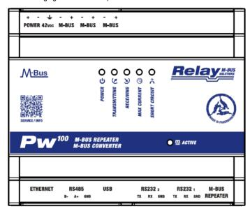
All terminals are pluggable and thus make wiring and replacement of the PW100 easier in the event of a fault.
