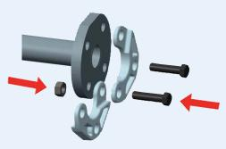
» Hold the 2 flange segments together and place two bolts in the two lower holes, fix the nuts by hand.
