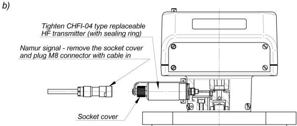
Fig. 17. Connection of the control element.
