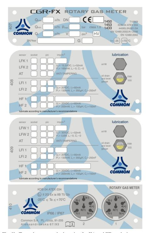
Fig. 8b. Type plates – standard version for IIA and IIB explosion groups
