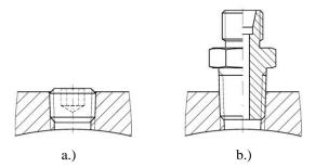
Fig. 6. 1/4" NPT pressure measurement tap
