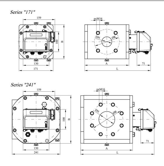
Fig. 14. Basic dimensions of CGR-FX rotary gas meters.
