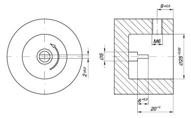
Fig. 7a Mechanical output drive shaft
