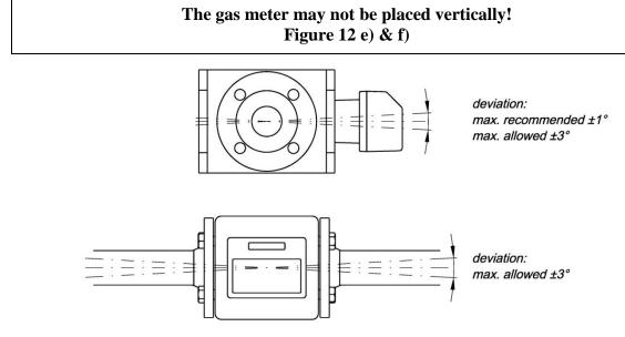
Fig. 13. Acceptable deviations from the horizontal position of the gas meter.
