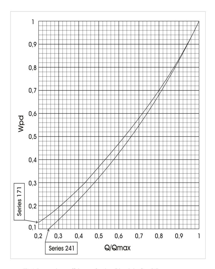
Fig. 1. Pressure drop coefficient as a function of the relative flow  $Q/Q_{\text{max}}$ .
