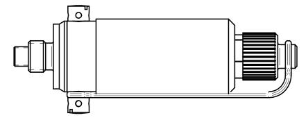
Fig. 19. CHFI-04 replaceable HF transmitter
