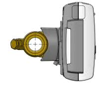
**Note:** In case of compact mounting, it may be necessary to use the enclosed angle fitting with some types of ULTRAFLOW® to obtain the required combination of viewing angle for the calculator's display and installation angle for ULTRAFLOW®.
