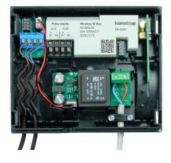
Wireless M-Bus-module with internal antenna
