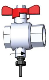
The composite union nut is tightened by hand. No tools must be used.
