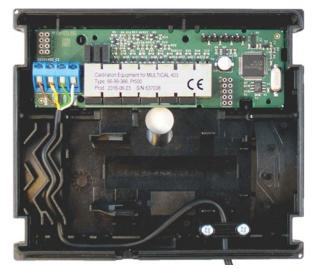
The calibration equipment comes in two different types, depending on the type of MULTICAL<sup>®</sup> 403 to be calibrated (Pt100 or Pt500). Both calibration equipments calibrate the meter as both heat meter and cooling meter via five calibration points.
