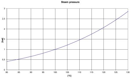
Diagram 2. Steam pressure as a function of temperature
