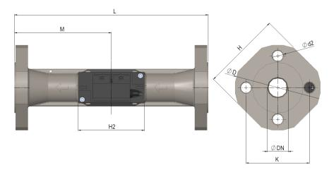
*Figure 12: Flow sensor with DN25, DN40 and DN50 flange connection* Flange facing type B, raised face in accordance with EN 1092-1, PN25
