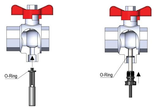
The O-ring duct is used for pushing the O-ring into place after which the temperature sensor can be pushed to the bottom.
