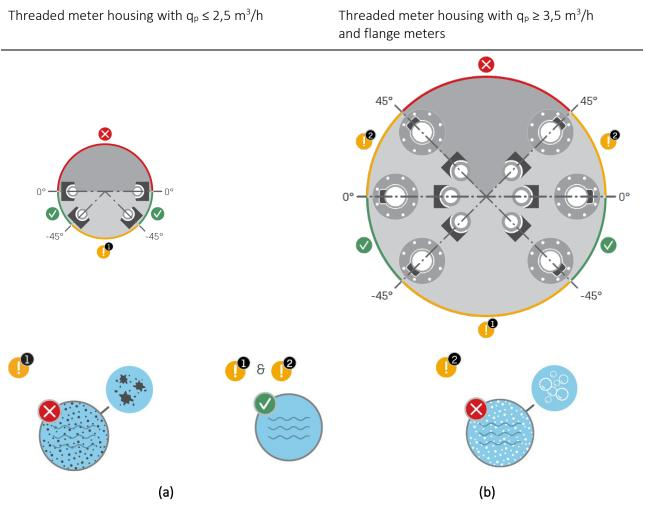
Figure 4. Acceptable orientation of Kamstrup flow sensors around the pipe axis for heating applications at horizontal mounting. (a) Threaded meter housings with  $q_p \le 2,5 \text{ m}^3/h$ . (b) Threaded meter housings with  $q_p \ge 3,5 \text{ m}^3/h$  and flange meters.
