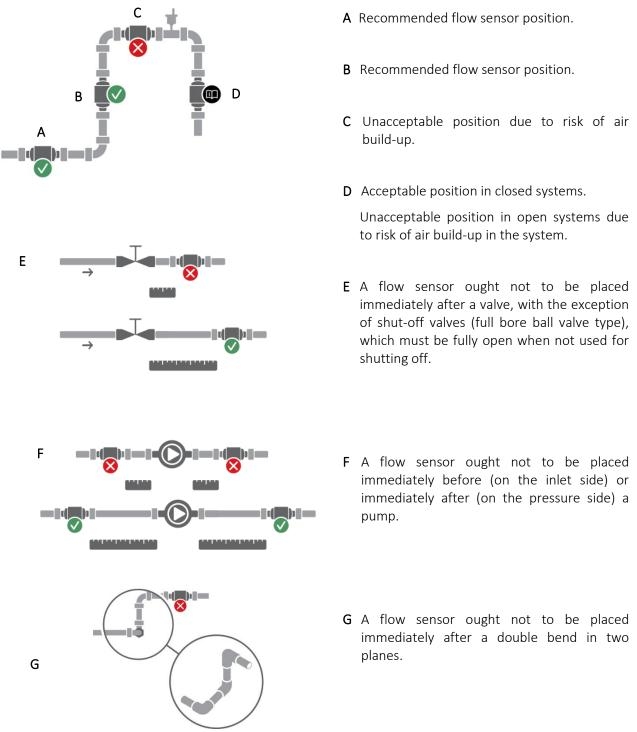
Figure 2. General installation recommendations for flow sensors.
