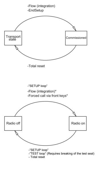
$^{*}\mbox{lf}$  the meter is in "TEST loop" the radio remains off at flow (integration) and forced call
