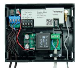
Wireless M-Bus-module with external antenna
