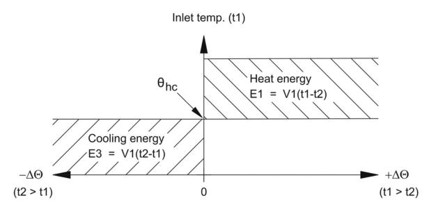
$\theta_{hc}$  acts as a limit value for the measurement of heat/cooling energy. With  $\theta_{hc}$  enabled, heat energy is only measured when t1 is greater than or equal to  $\theta_{hc}$ . Likewise, cooling energy is only measured if the inlet temperature t1 is lower than  $\theta_{hc}$ .
