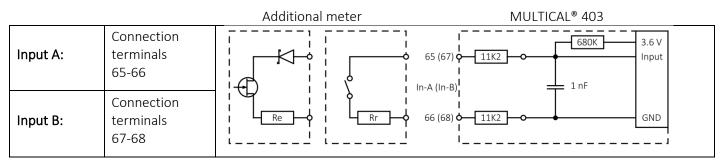
The pulse inputs are configured as a part of the meter's configuration number via the FF- and GG-codes. Upon receipt of order the FF- and GG-codes are configured at 24 by default (unless otherwise informed by the customer). Valid FF- and GG-codes appear from the table below. The default code 24 is marked in green. The FF- and GG-codes can be reconfigured by means of the PC-program METERTOOL HCW. See Technical description for METERTOOL HCW (5512-2097).
