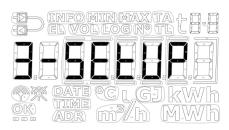
In this loop the technician can configure the meter via the front keys. This enables the technician to configure the meter both before installation and after commissioning of the meter. Configuration of the meter after commissioning requires that the installation seal is broken and that meter top is separated from meter base.
