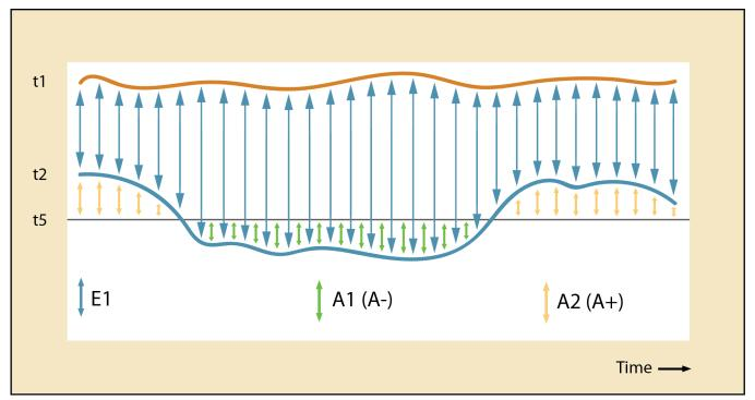
The outlet temperature reference t5 can be factory-configured as required, or can be changed via METERTOOL HCW after delivery. Typical configuration is t5 = 50  $^{\circ}$ C.
