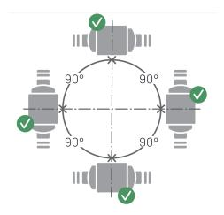
Kamstrup's flow sensors can be mounted vertically, horizontally or at an angle.
