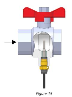
To obtain the best possible serviceability during meter exchange, the direct short sensor can be placed in a ball valve with sensor socket, see *Figure 15*.
