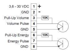
When Pulse Interface type 6699-143 is connected to power supply or battery, the unit is placed on the meter, and the meter is in test mode, the following pulses are transmitted:
