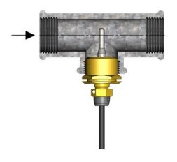
As it appears from *Figure 14*, the direct short sensor DS 27,5 mm can be mounted by means of a  $R\frac{1}{2}$  or  $R\frac{3}{4}$  for M10 nipple in a standard 90° tee.
