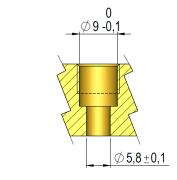
Figure 16: Measurement and tolerance requirements when installing a direct Ø5.0 mm or Ø5.2 mm temperature sensor.
