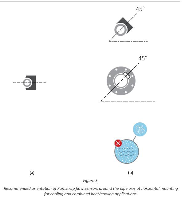
(a) Threaded meter housings with  $q_p \le 2,5 \text{ m}^3/h$ . (b) Threaded meter housings with  $q_p \ge 3,5 \text{ m}^3/h$  and flange meters.
