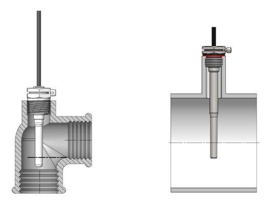
Figure 17: Examples of installation of sensor pocket for Ø5.8 mm temperature sensor with R½ thread (to the left) and sensor pocket for Ø6.0 mm temperature sensor with G½ thread and copper gasket (to the right).
