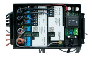
Wireless M-Bus-module with internal antenna
