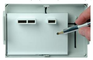
The contact pads must be shorted while the calculator top is still active (display on). If it is not possible to keep the calculator top active, the recommendation is to remove the communication modules from the base, assemble the calculator and then open the calculator again and short the contact pads.
