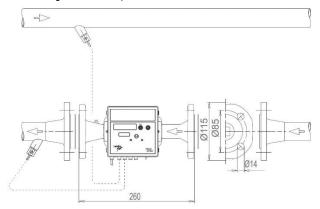
Fig. 10: Installation with pockets (recommended greater than or equal to qp 10)
