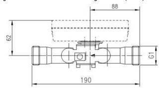
Fig. 3: Overview dimensions overall length 190 mm (thread)
