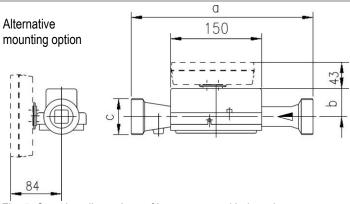
Fig. 5: Overview dimensions of large meters with thread
