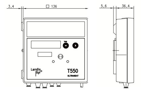
Fig. 15: Dimensions of electronic unit
