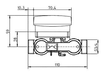
Fig. 1: Overview dimensions overall length 110 mm
