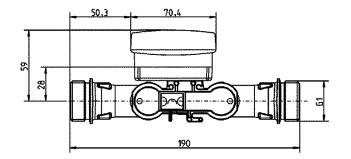
Abb. 3: Overview dimensions overall length 190 mm (thread)
