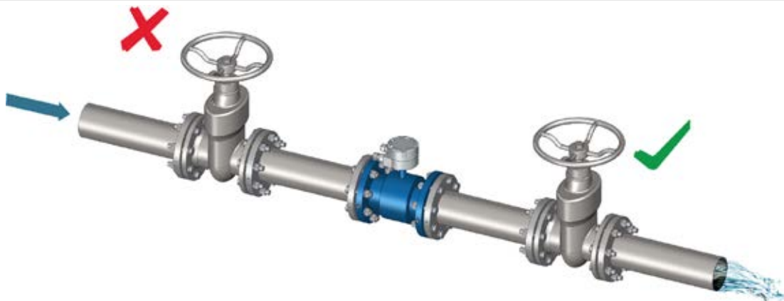
Fig. 35 | Gate valves installation
