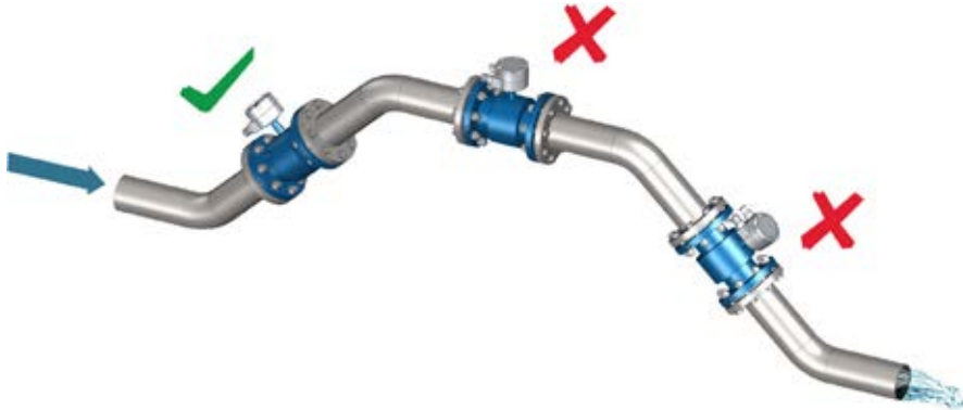
Fig. 34 | Correct (LH) and incorrect installation (central and RH)
